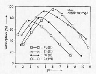
Figure 4. Effect of pH on the adsorption of chemically activated sawdust
